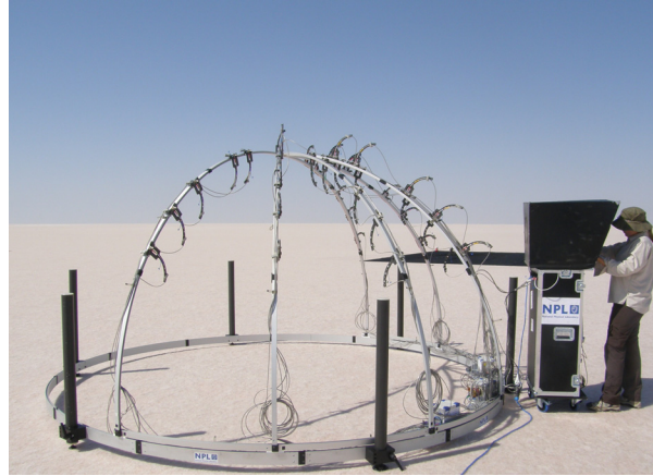
Figure 4: The NPL Gonio Radiometric Spectrometer System (GRASS) conducting measurements on Tuz Gölü, Turkey, August 2008.
